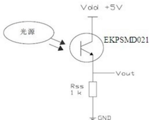
注：光电流 =  $V_{out} / R_{ss}$
